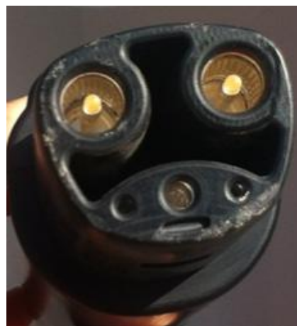
Fig.2 Tesla Supercharger fast DC plug. [8]
