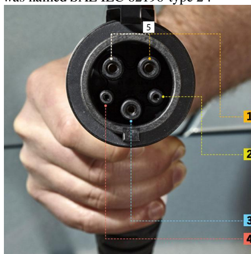
Fig.1 SAE J1772-2009 AC US plug, (1-L1; 2-PP; 3-PE; 4-CP; 5-N) [3]
